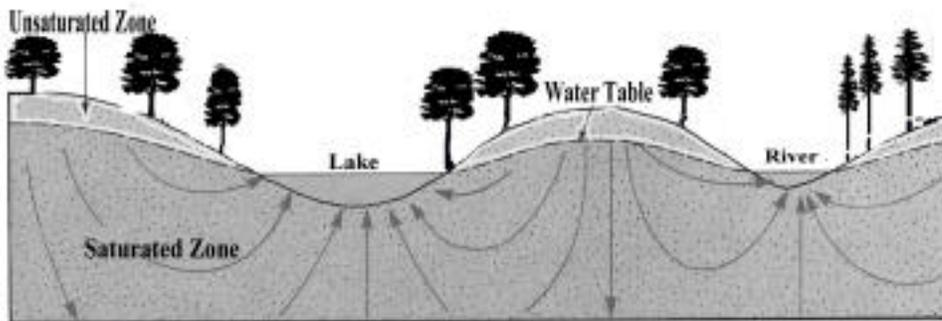
**Figure 6. Relationship between groundwater and surface water.**
